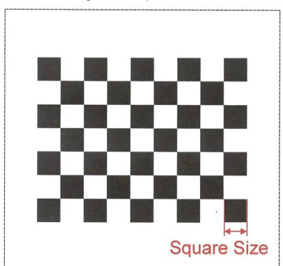
· Rows and Columns are the connection points of the black squares. The correct number is 8 for columns and 6 for rows
