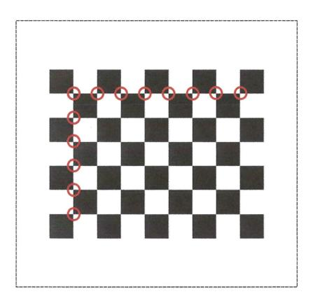
• Origin Distance is the distance between turntable surface and the upper edge of the black squares in the row close to the turntable.
